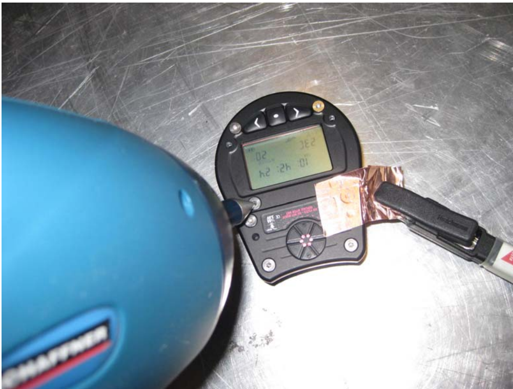
Photo 4.1.8 Test setup regarding immunity to electrostatic discharges.
