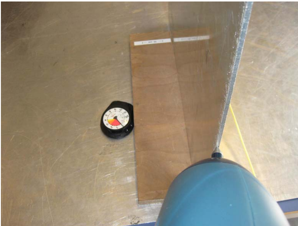
Photo 4.1.2 Test setup regarding immunity to electrostatic discharges.
