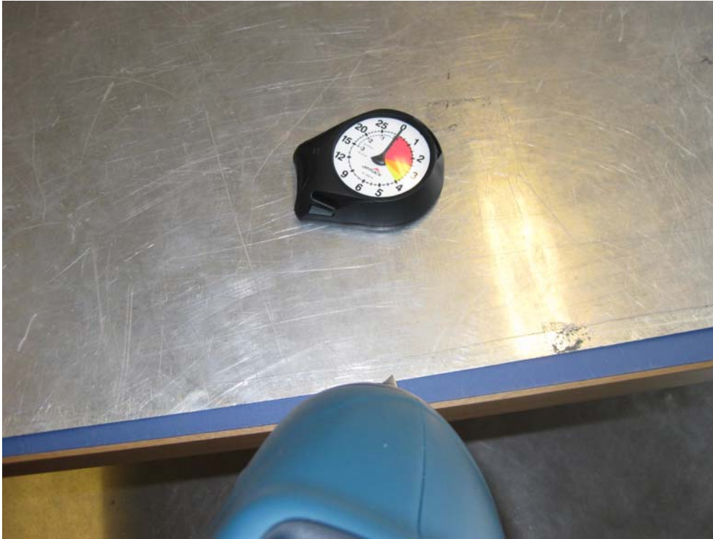
Photo 4.1.1 Test setup regarding immunity to electrostatic discharges.
