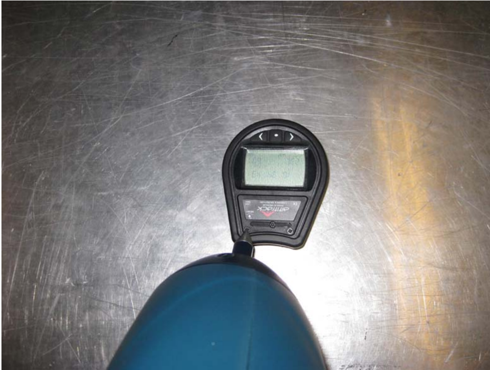
Photo 4.1.3 Test setup regarding immunity to electrostatic discharges.
