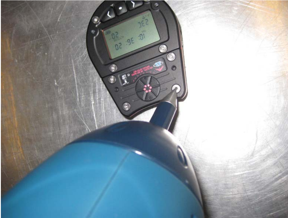
Photo 4.1.7 Test setup regarding immunity to electrostatic discharges.
