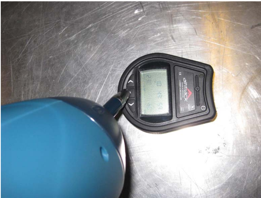
Photo 4.1.4 Test setup regarding immunity to electrostatic discharges.
