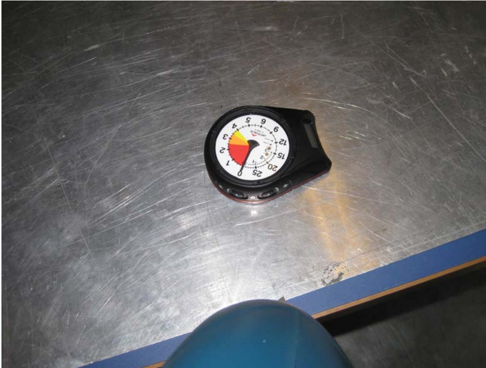
Photo 4.1.5 Test setup regarding immunity to electrostatic discharges.
