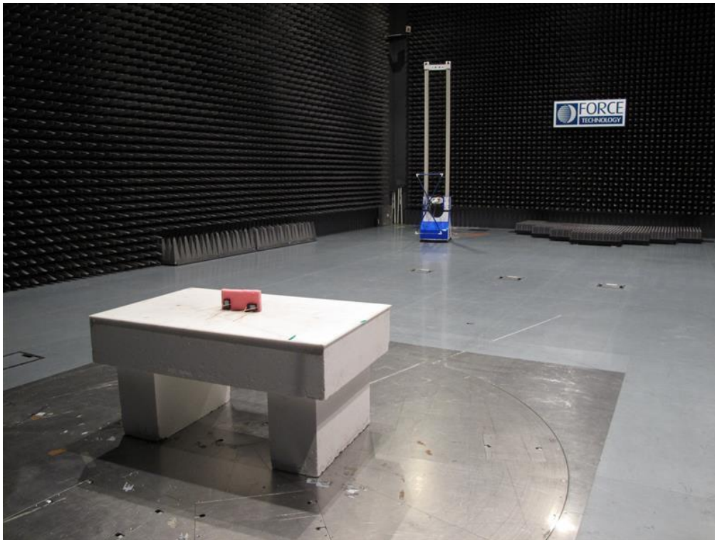
Photo 4.1.1 Test set-up regarding measurement of radio frequency electromagnetic field.
